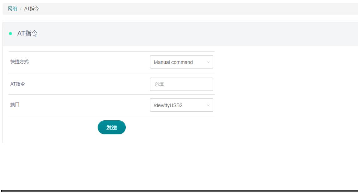
The screenshot shows a web-based interface for sending AT commands. The top navigation bar says "网络 / AT指令". Below it, a section titled "AT指令" is selected. There are three input fields: "快捷方式" (set to "Manual command"), "AT指令" (marked as required), and "端口" (set to "/dev/ttyUSB2"). A blue "发送" (Send) button is at the bottom.
