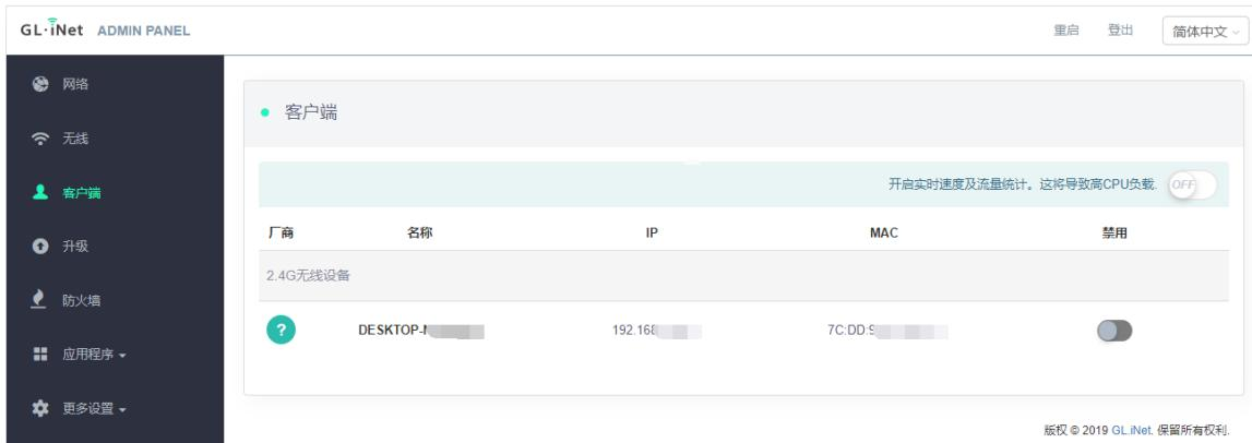
The screenshot shows the GL.iNet Admin Panel interface. On the left is a sidebar with icons for Network, Wireless, Clients, Upgrade, Firewall, Applications, and More Settings. The main panel is titled '客户端' (Clients) and lists a single device: 'DESKTOP-1' with IP '192.168.1.10'. There is a toggle switch for '禁用' (Disable). A note at the top right says '开启实时速度及流量统计。这将导致高CPU负载。 OFF'.
